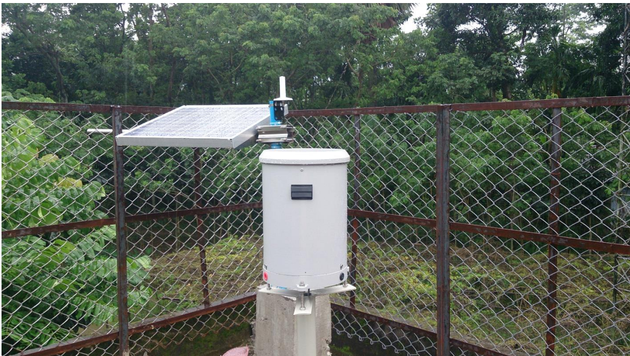
Figure 7: Tipping Bucket and Solar Panel on the roof of gauge house
