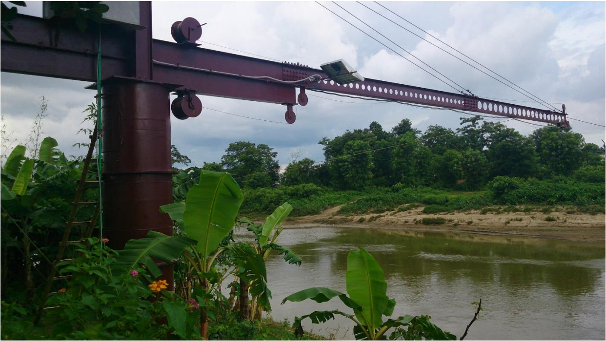
Figure 1: Metal Structure for Mounting Radar Level Sensor
