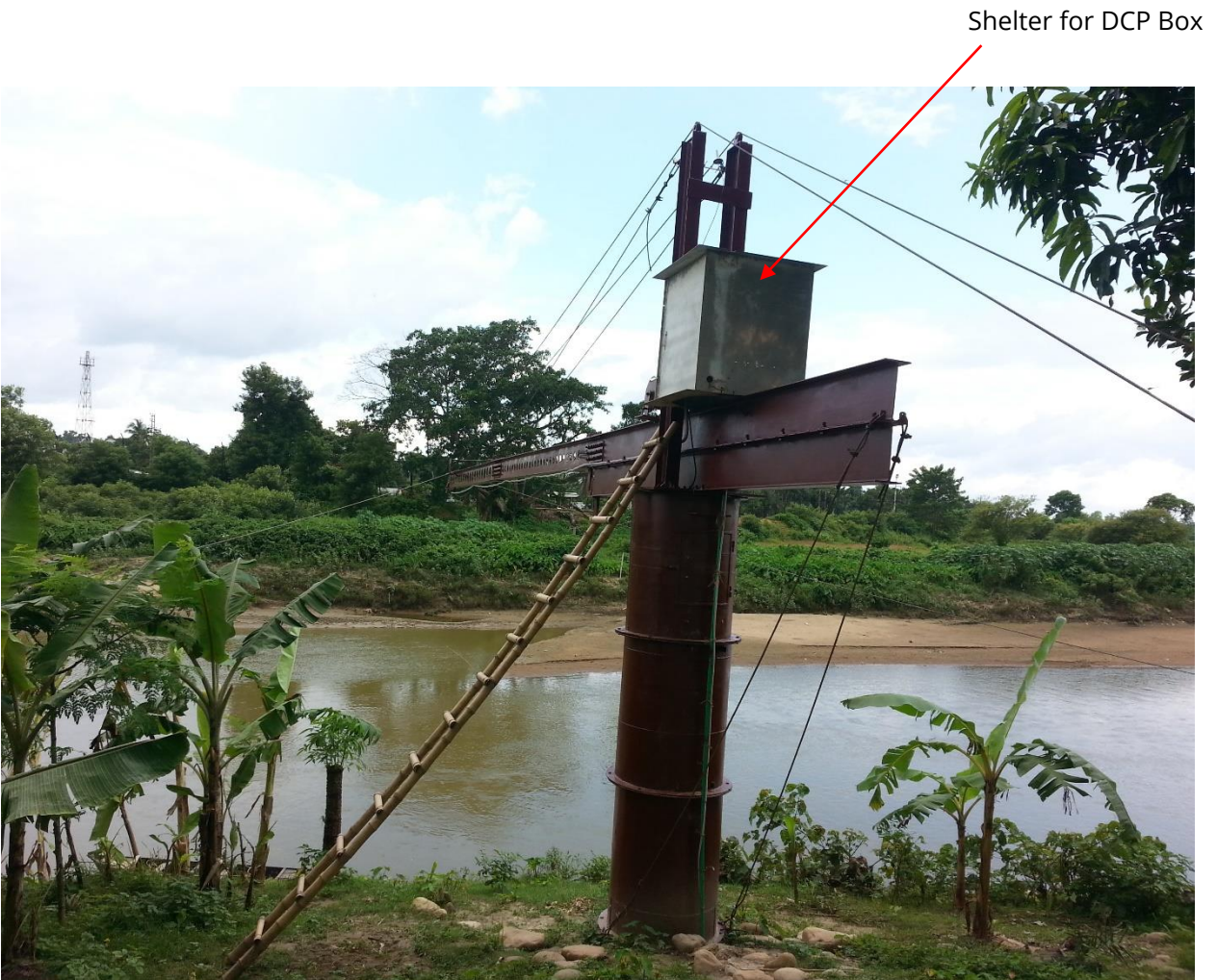
Figure 1: Metal Structure for Mounting Radar Level Sensor
